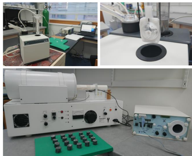
Fig. 3 The M 3 Ore Lab is equipped with (top left) a KLY-5a Kappabridge with CSL cryostat and CS4 Furnace, (top right) a 3D automated rotator, and (bottom) a selection of hand held susceptibility meters, an impulse magnetiser, isothermal demagnetiser, and Molspin magnetometer.
